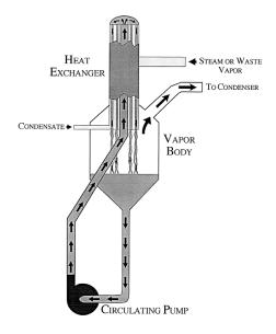
Liquid and vapor from the heat exchanger tubes enter the vapor body directly for vapor separation. A circulating pump is required to maintain proper evaporator liquid flow.
