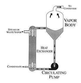
The liquid and vapor leave the heat exchanger together and enter the vapor body. After vapor separation the evaporator liquid flows from the vapor body through the circulating pump to the heat exchanger.
